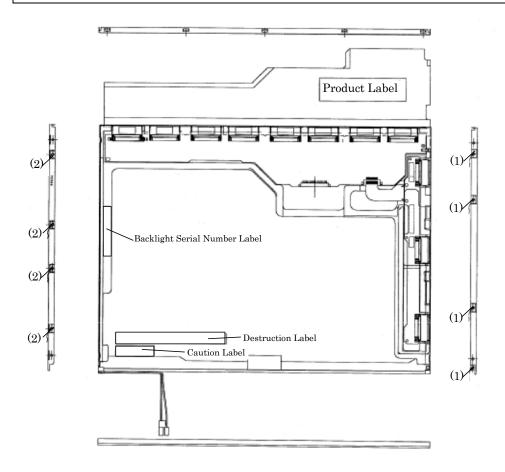
Figure 4-52 Replacing TMD fluorescent lamp (WXGA) (2)
